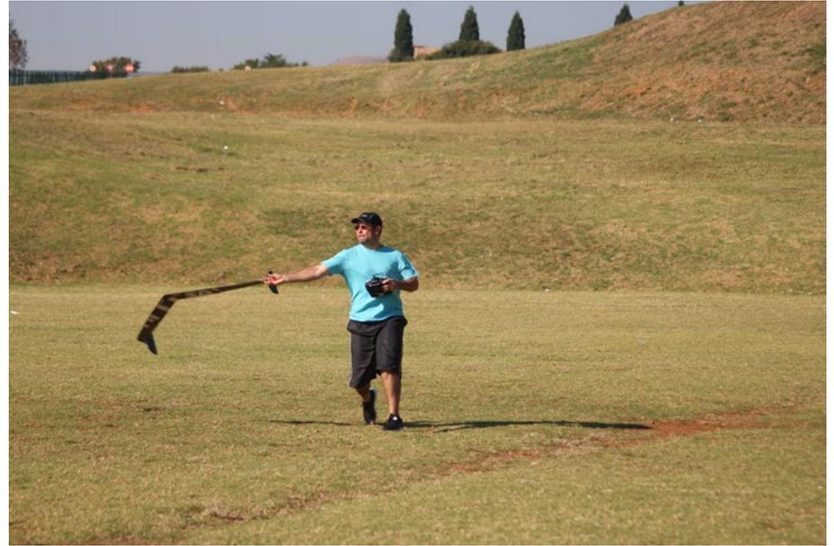
The slope version can also be used on a flat field and launches higher than the thermal version, but due to the heavier wing loading it makes it harder to catch thermals.
